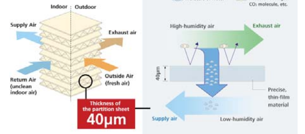
Principle of ERV system
