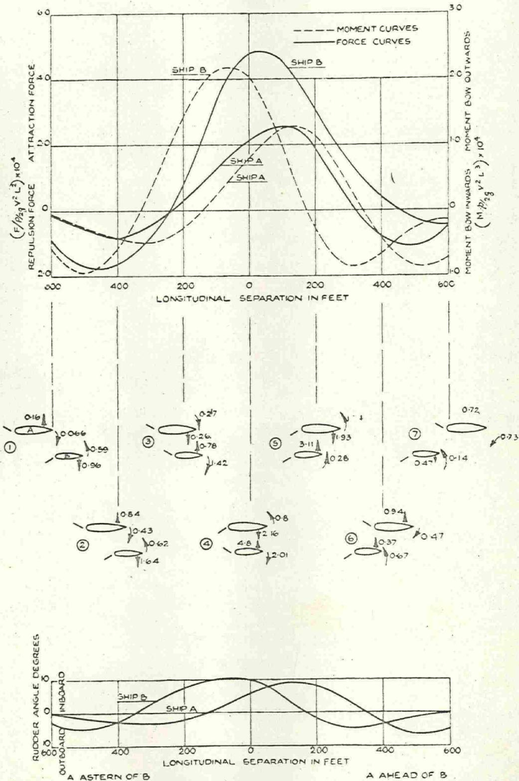
Fig. 2.—Measured Interaction Forces and Moments and Correcting Rudder Angles (100-ft. Separation Beam-to-beam).
