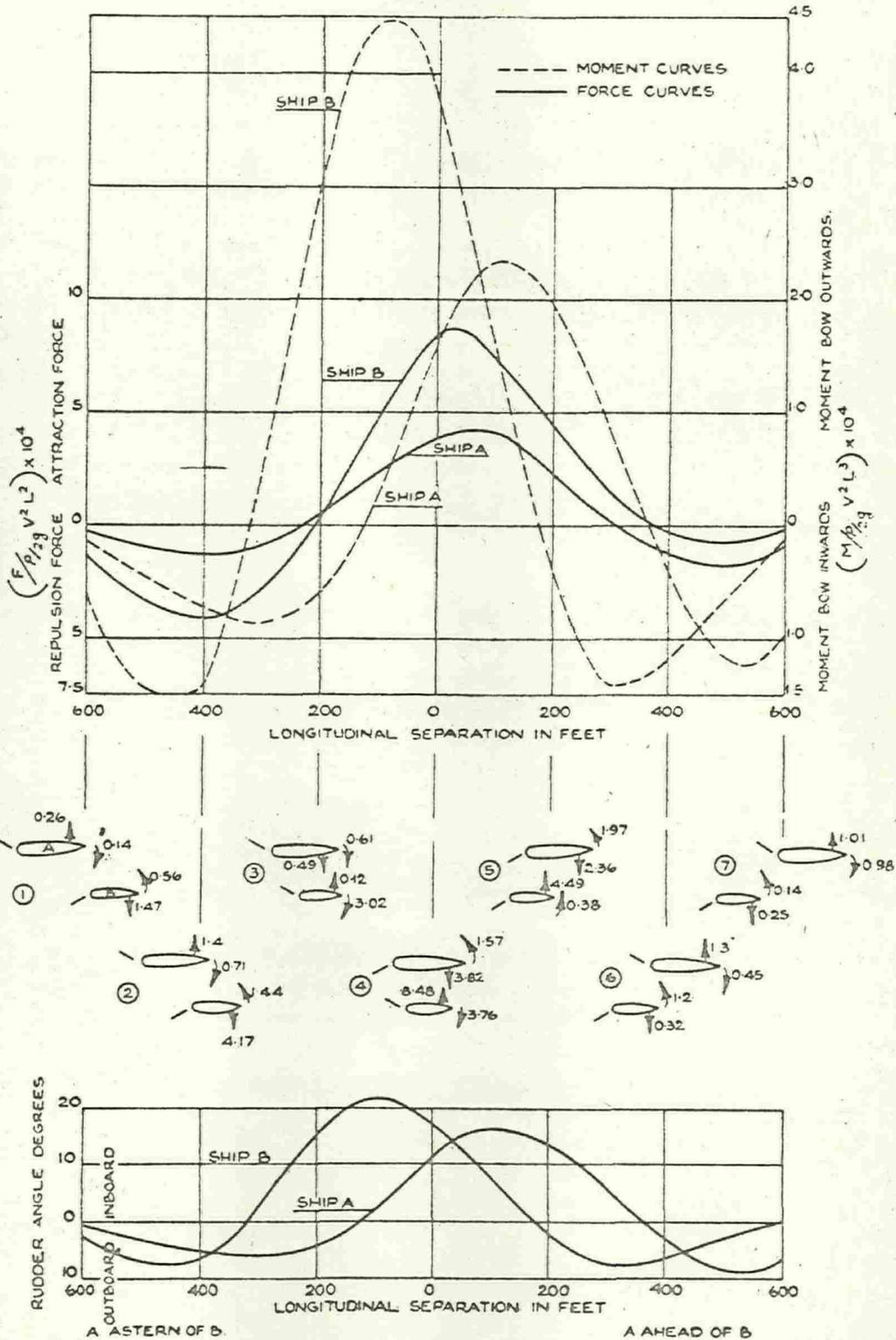
Fig. 1.—Measured Interaction Forces and Moments and Correcting Rudder Angles (50-ft. Separation Beam-to-beam).
