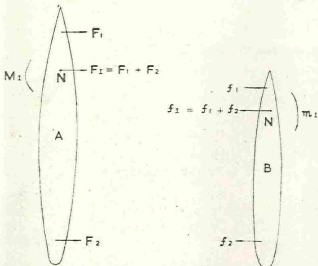
Fig. 3.—Forces and Couples Due to Interaction.
