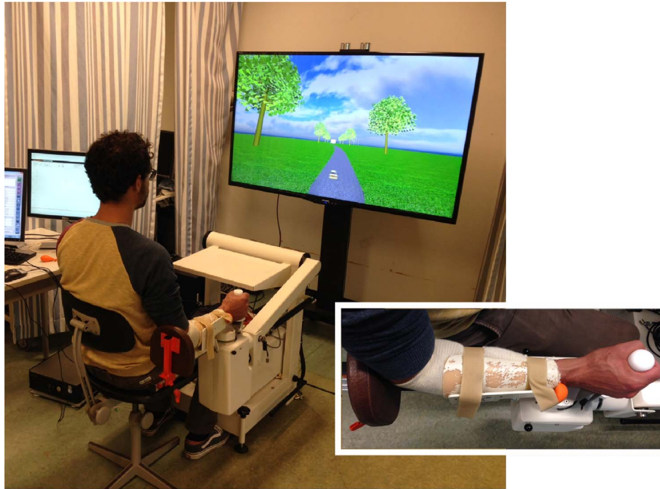
Fig. 1. Overview of the experimental setup, with a close-up top view of the arm positioned in the haptic robot.
