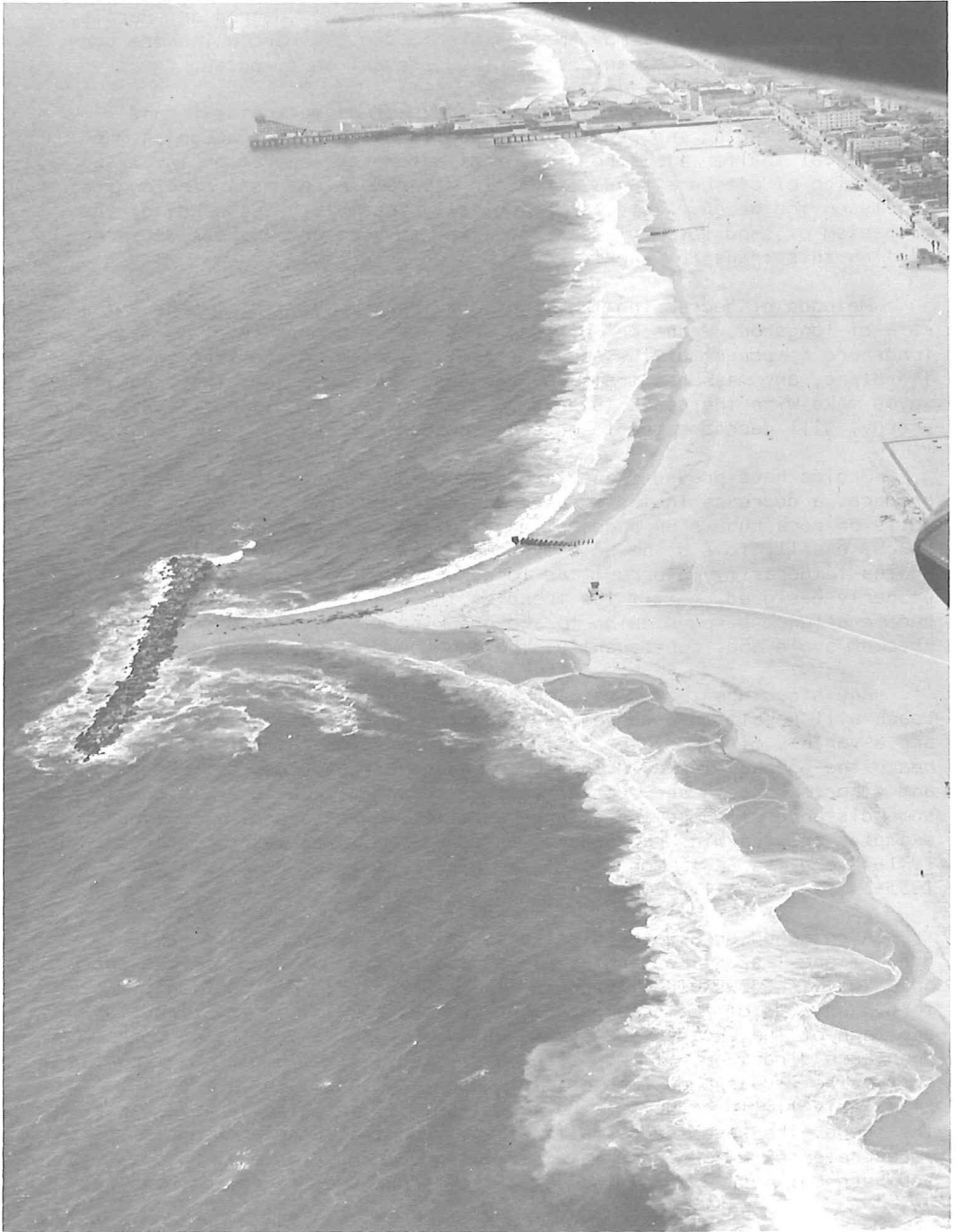
Figure 6. Aerial photograph of a breakwater at Venice, Santa Monica Bay, California. Wave shadow in lee of breakwater has caused a tombolo to form joining breakwater to the beach.
