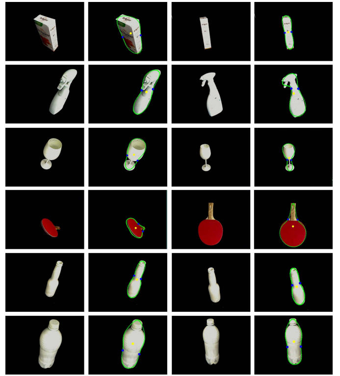
Fig. 14. Snapshots from the experiments. First and third columns are the initial views and the views obtained after the viewpoint optimization, respectively. Second and forth columns present the elliptic Fourier descriptors (EFD) model and synthesized grasping points for these views; the green points represent the EFD model, the yellow points are the centre of the models [(a_0, c_0)] points], and the blue points are the grasping points. Comparing the initial viewpoints with the final one, it can be seen that, the viewpoint optimization does not only help the grasping synthesis algorithm to generate better grasping points, but it also provides good approach vectors for the grasp execution.
