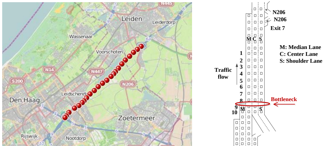
Figure 2.3: Open street figure of targeted section in freeway A4 in the Netherlands (left) shown in red dots and the layout of the study site (right). The bottleneck is a lane-drop bottleneck highlighted with a red circle. This chapter only targets 10 locations. The total distance from the location 1 to location 10 in the freeway is approximately 4.5 km. The bottleneck is around 6.5 km away from the downstream off-ramp.
