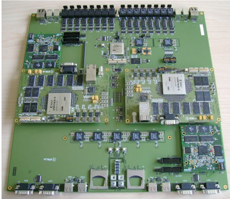
Figure 3.3: Picture of the hArtes Hardware Platform. The two BCEs use two daughters boards each, one for the D940HF processor and one for the FPGA based infrastructure. The ADAT interfaces and several standard I/O connectors are clearly visible at the top and at the bottom of the picture, respectively. [83].
