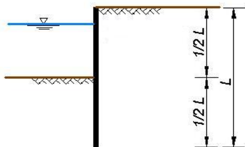
Figure 2.8: Freestanding sheet piling
