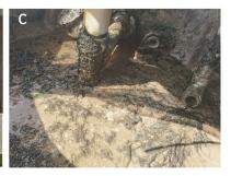
**Figure 4.3.** Deposits in the basin of the reference (a), P-limited (b) and non-P-limited (c) cooling towers at the end of the 5-week experiment.
