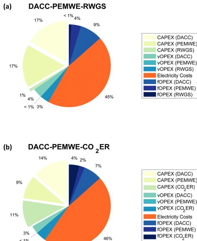
Fig. 5 The percentages of CAPEX, variable OPEX, electricity costs, and fixed OPEX of each technology for (a) DACC-PEMWE-RWGS and (b) DACC-PEMWE-CO<sub>2</sub>ER pathways. Exploded: CAPEX fractions. Non-exploded: OPEX fractions. Note that the vOPEX percentage excludes electricity costs, which has its own contribution.
