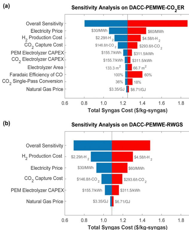
Fig. 6 Sensitivity analysis on technical and economic metrics for (a) DACC-PEMWE-RWGS and (b) DACC-PEMWE-CO<sub>2</sub>ER.
