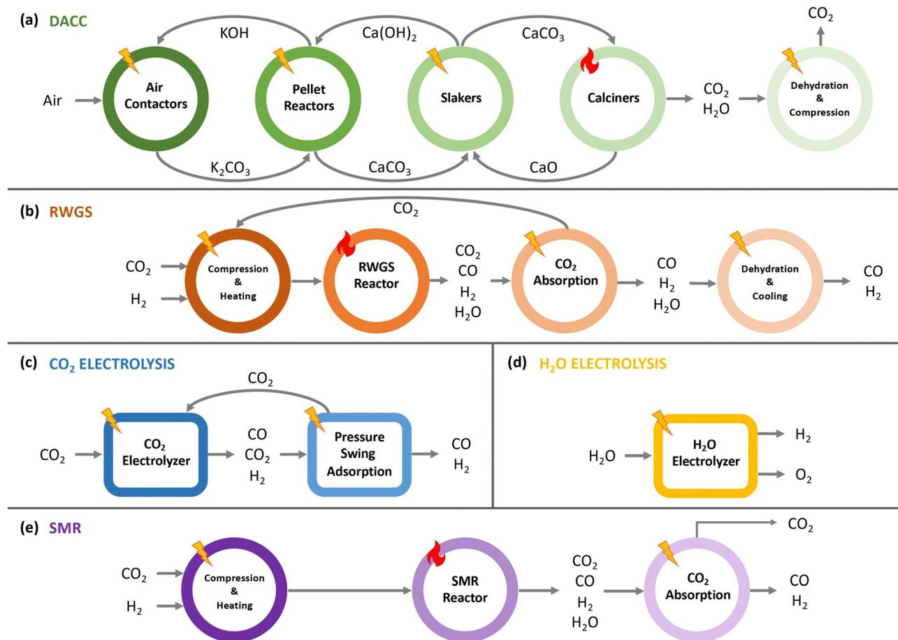
Fig. 1 Simple block flow diagrams of (a) liquid hydroxide-based DACC, (b) reverse water gas shift, (c) CO<sub>2</sub> electrolysis, (d) H<sub>2</sub>O electrolysis, and (e) steam methane reforming. The fire symbol represents fossil-based thermal energy and the lightning bolt symbol represents electricity, which can be sourced from renewables.
