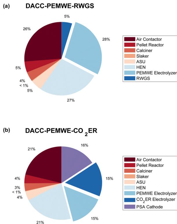
Fig. 4 ISBL cost breakdown structure of (a) DACC-PEMWE-RWGS and (b) DACC-PEMWE-CO<sub>2</sub>ER, showing the percentages of cost components. Exploded: electrolyzers.
