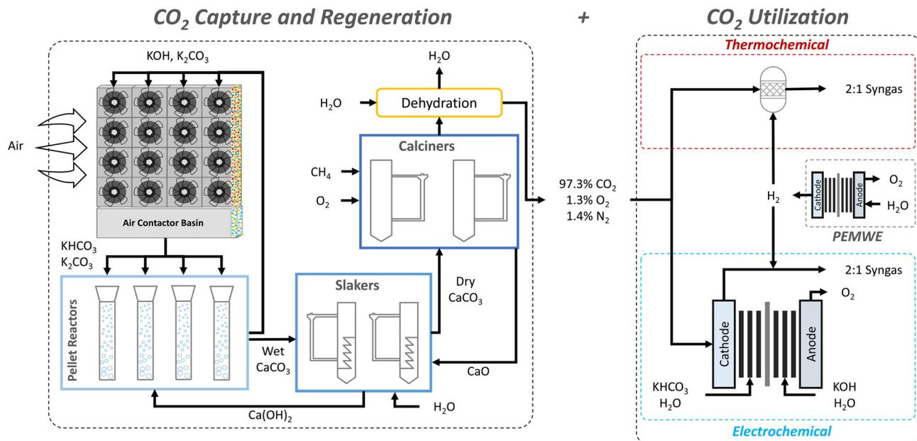
Fig. 2 Process flow diagram of the investigated pathways, exhibiting the integration of hydroxide-based DACC with RWGS and with the CO<sub>2</sub>ER. The yellow-colored monolith in the air contactors represent KOH wetting. The percentages of the CO<sub>2</sub> stream are based on mass.
