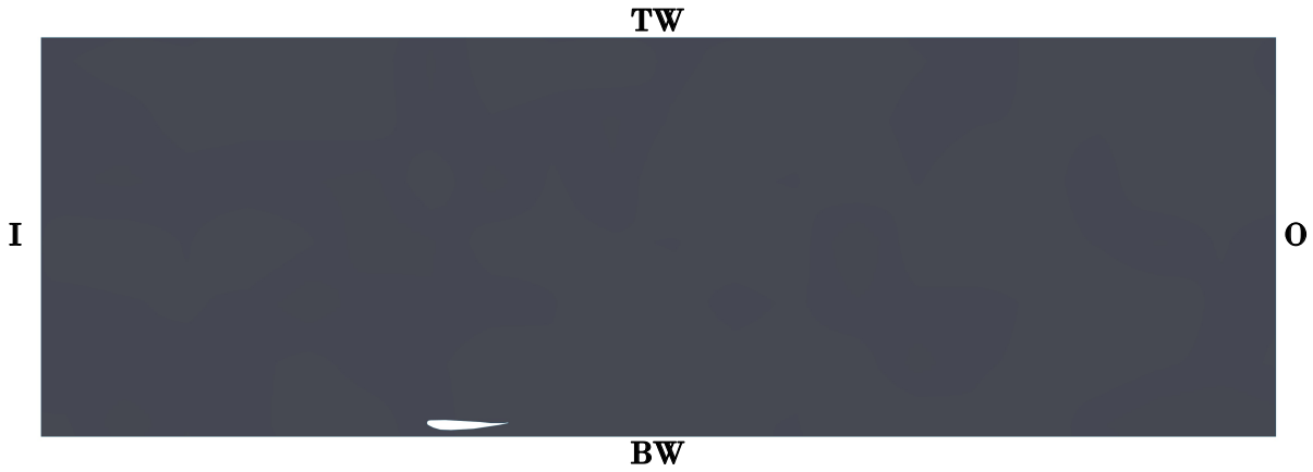
Figure 2.1: 2D computational domain for the Tyrrell 026 airfoil. I: Inlet, O: Outlet, TW: Top Wall, BW: Bottom Wall. The airfoil is positioned near the ground to investigate ground-effect behavior
