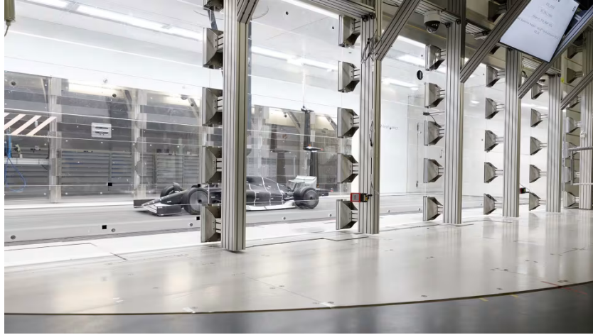
Figure A.1: A 60% scaled model of a F1 car tested in a Wind tunnel [Formula 1, 2024b]
