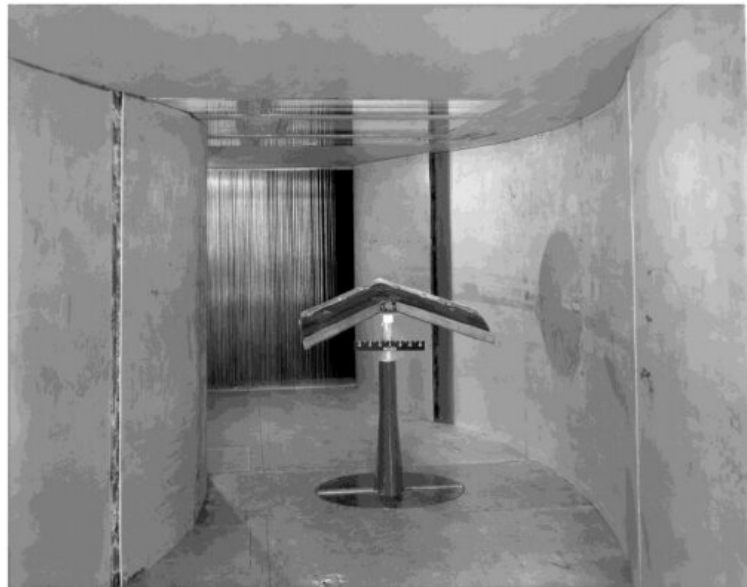
Figure A.9: Inside View of the Langley Stability Tunnel Curved Test Section [Keogh, 2016; Keogh, Barber, et al., 2015]
