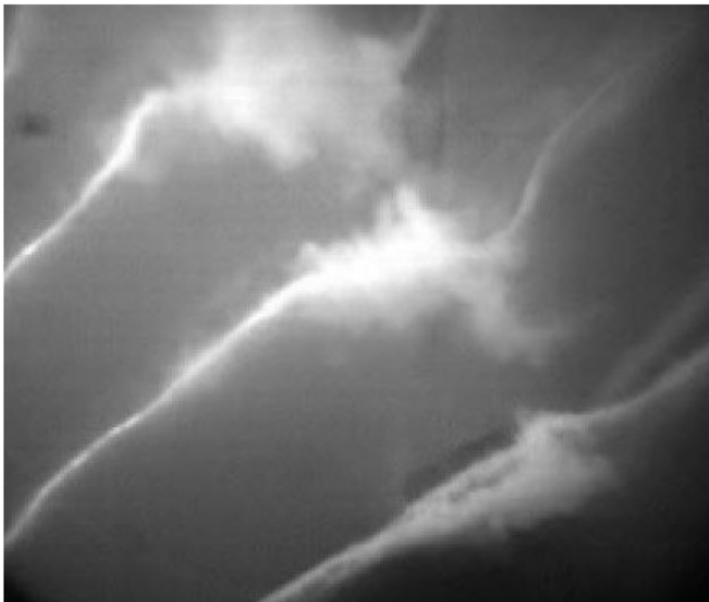
Figure 2-9: Visualization of the breaking up tip vortex cavitation (Friesch, 2006)
