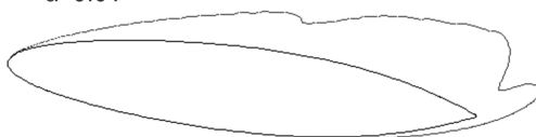
Figure 6-48: Contour of vapor fraction with iso-value of 0.01 at the instant ⑥ in Figure 6-47
