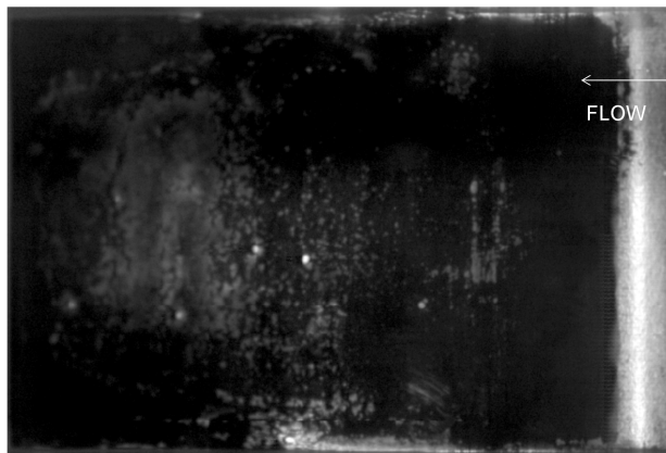
Figure 8-1: Paint test result after re-application of paint and run No.26 and 27 ( \sigma = 2.01 , U = 17.3m/s ) on a NACA0015 hydrofoil at 8^\circ angle of attack (30 – 60 minutes)
