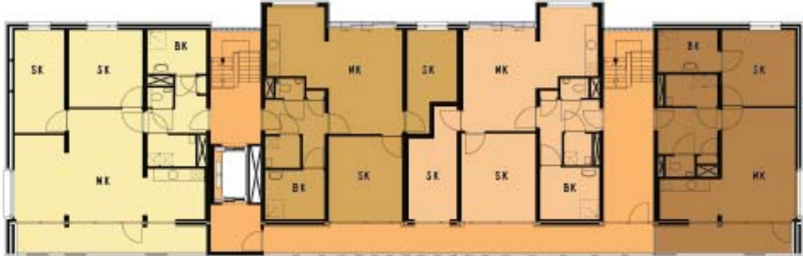
Internal walkway with elevator and staircases
