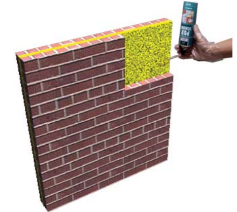
Adding insulation by 'parging' cavity walls
