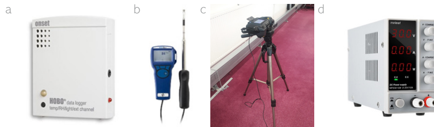
Figure 31. a: Datalogger (HOBOT), b: air velocimeter, c: infrared camera, d: power supply
