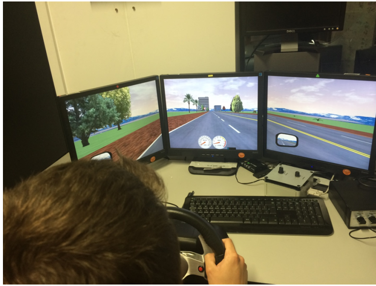
Figure 1 Driving simulator used in Experiment 1. The photo illustrates the hardware setup; the virtual environment in the actual experiment was not identical to the one shown in the figure (see online version for colours)
