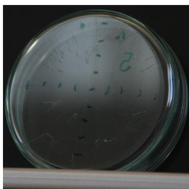
(e) 12.5 % Topas 5013 in Toluene,  $\omega_1=5000$  rpm,  $\alpha_1=400$  rpm/s,  $t=50$  s
