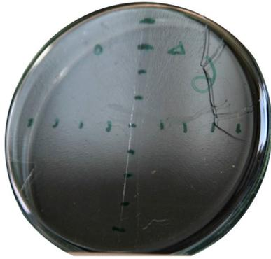
(a) Result of sample 6 from experiment 1,  $\omega_1 = 3900$  rpm. Along the centre of the petri dish the TOPAS film is scratched away to allow for thickness measurements. The surface is not smooth but shows radial ripples.
