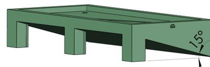
Figure B.3: Model of the printed mold. The bottom is tilted with  $15^\circ$  to advance drainage of the resin to the side.
