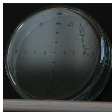
(f) 12.5 % Topas 5013 in Toluene,  $\omega_1=3900$  rpm,  $\alpha_1=250$  rpm/s,  $t=50$  s
