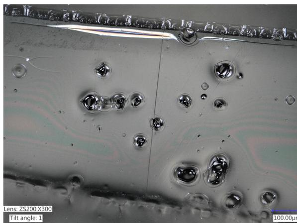
Figure 3.8: Spherical defects in the spin coated TOPAS layer on top of the sputter coated Au/Pd line. Picture made with a confocal microscope, 300 $\times$  magnified.
