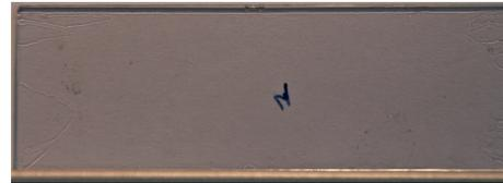
(b) Result of sample 4 of experiment 2,  $\omega_1 = 3900$  rpm. The surface is smooth, no defects visible for the naked eye. Irregularities along the edges are caused by insufficient wetting of the surface.
