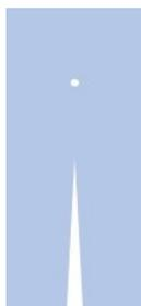
Figure 3.1: PDMS mask (17x38 mm) applied for sputter coating Au/Pd on TOPAS 6015 substrates.
