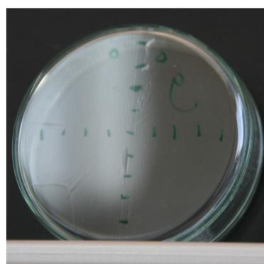
(i) 12.5 % Topas 5013 in Toluene,  $\omega_1=2000$  rpm,  $\alpha_1=100$  rpm/s,  $t=50$  s
