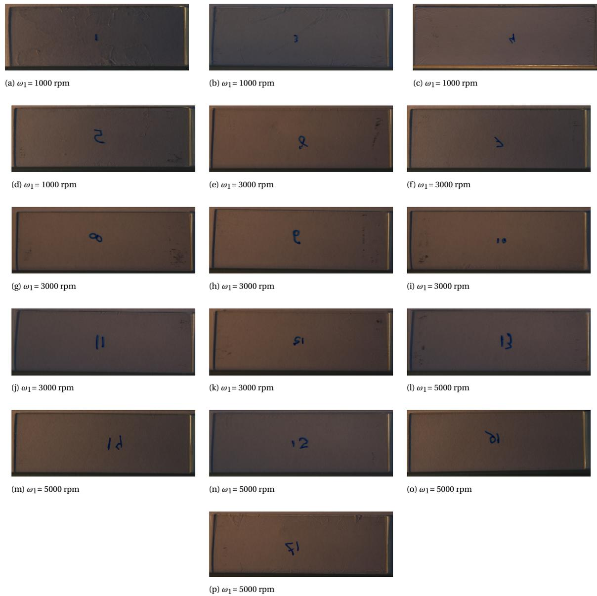
Figure D.4: Spincoating results of dissolved 25wt% Topas 5013 in sec-butylbenzene. Along the center of the microscope slides the Topas film is scratched away to allow for thickness measurements. Velocity of the first spincoating step is varied, acceleration is kept constant at  $\alpha_1 = 250$  rpm/s. The second spincoating step has been kept constant at  $\omega_2 = 100$  rpm and  $\alpha_2 = 250$  rpm/s
