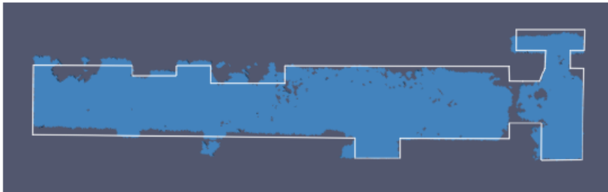
Figure 12: Comparing the navigable space generated from a point cloud to a floor plan (Staats et al., 2017)
