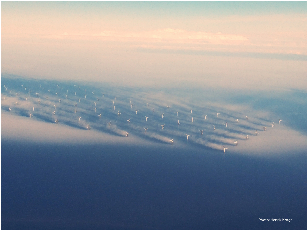
Figure 1-1: The flow patterns formed by the wake effect in Horns Rev 2 offshore wind farm in Denmark. A wake with lower kinetic energy and higher turbulence level is formed behind a turbine, and overlap with a downstream turbine. The picture was captured by Henrik Krogh.
