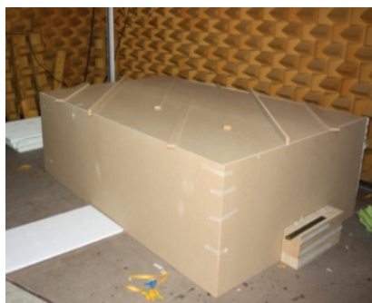
Figure 19 – Measurement setup of the 'closed box'.
