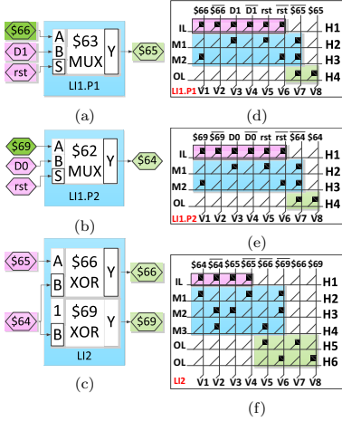
Figure 5: (a),(b),(c) Partitioned logic islands (d),(e),(f) Memristor crossbar layouts
