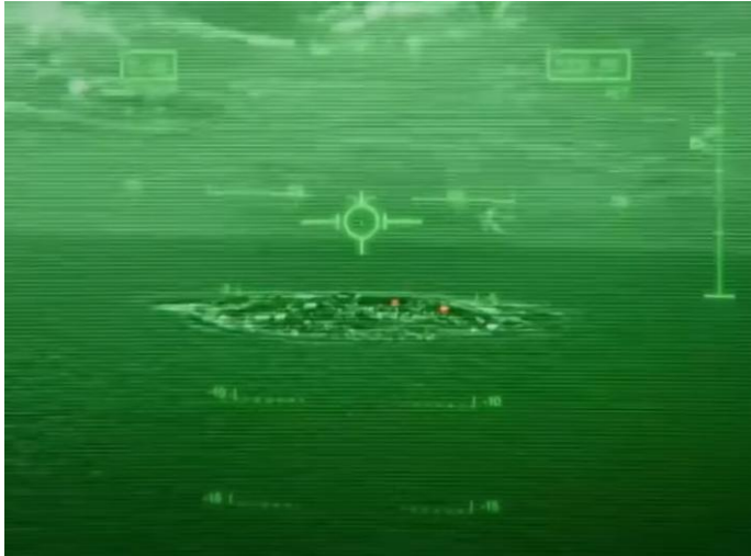
Figure 11: In-helmet HUD avionics and see-through plane night vision as displayed to the pilot (Joint Strike Fighter F-35 | Helmet Mounted Display System, n.d.).
