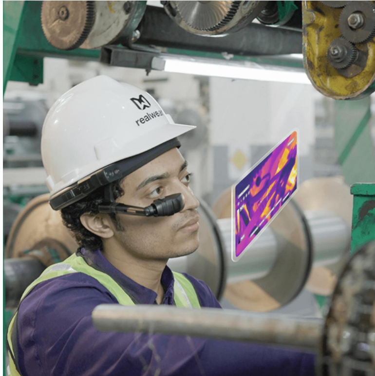
Figure 17: Realwear uses a relatively simple display technology that does not fully block the user's FOV, ensuring normal peripheral vision and safety (RealWear Navigator 520 | Devices, n.d.).
