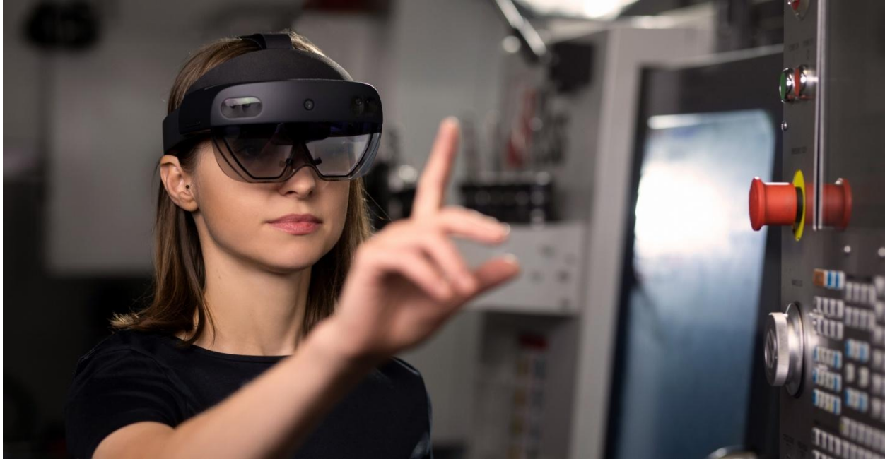
Figure 16: The Microsoft HoloLens 2 was specifically aimed at enterprise and industrial use, featuring some ruggedness such as IP50 dust-proof rating, hardhat compatibility and operability with gloves (Jowita Kessler, 2022).
