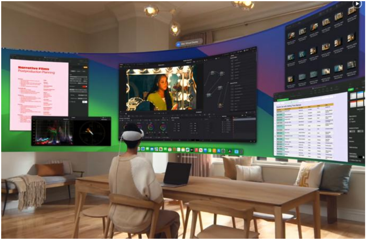
Figure 13: Apple Vision Pro user experience in “2D” AR mode: You can use it as a very high definition (12 MP per eye (4K = 8MP)), ultra-wide monitor to enhance your work space where screen real estate is projected over your entire field of view, while still showing the real environment. Works standalone or enhances phone / laptop workspace. This is one of the more ‘traditional’ workflows offered by the system, enhancing the user experience people are already accustomed to (i.e. computing on a large screen) (Apple Vision Pro, n.d.).
