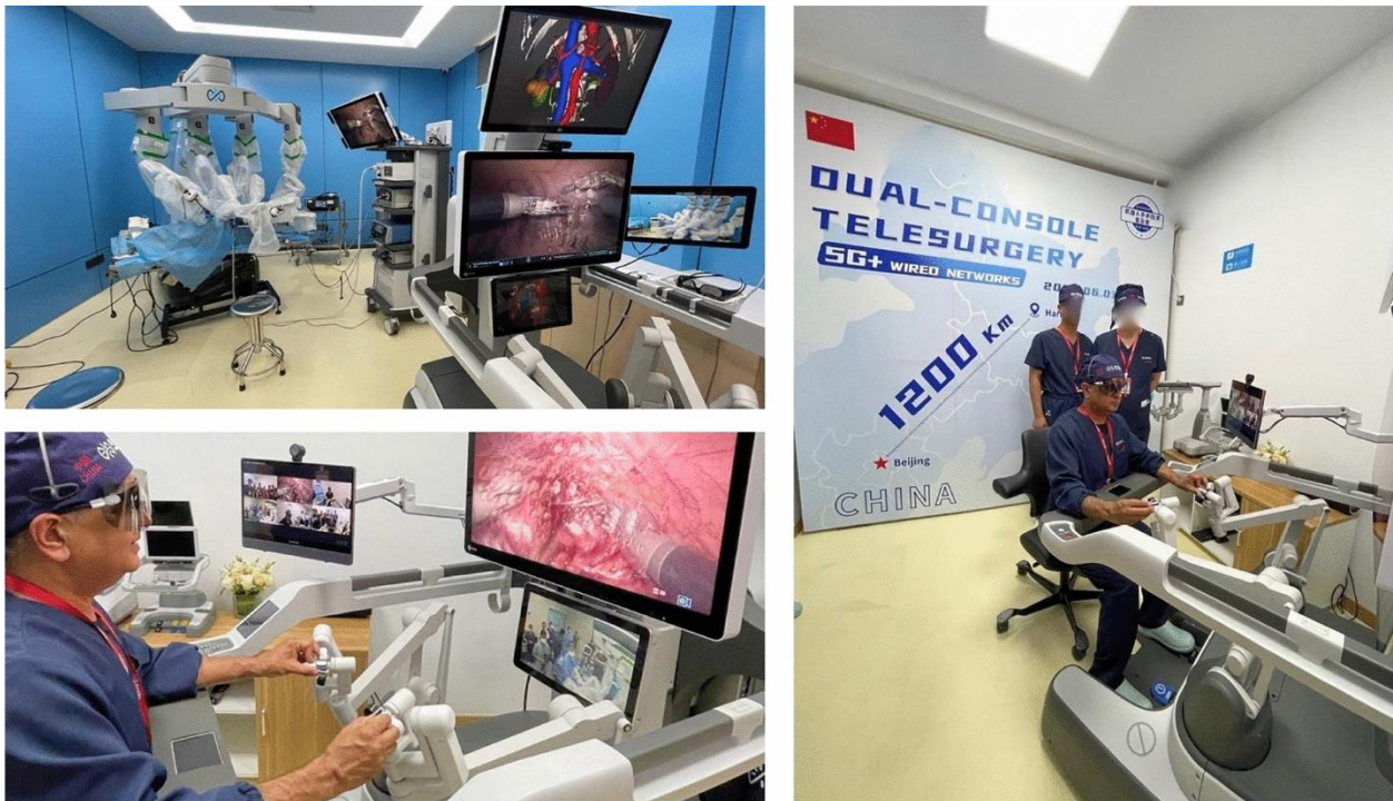
Figure 12: Telesurgery on an animal, spanning a 1200km distance in China, enabled by high-speed, low-latency (5G and fibre optic) networks. A surgeon console with operating room and control room views allows a doctor to remote control a surgical robot (Patel et al., 2024).
