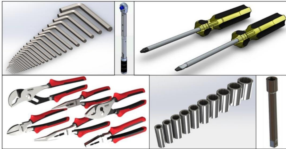
Figure 22: CAD models of not only the machines and parts, but also the tools used are required for creating digital field workflows and trainings (Mourtzis et al. (2020)).
