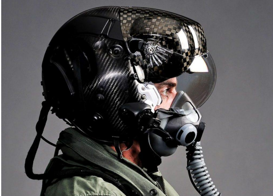
Figure 10: F-35 pilot wearing a custom-fit helmet, which has integrated AR capabilities for flight information, 360-degree visibility and sensor integration, demonstrating AR's usefulness in a high-profile use case (Schradin, 2022).
