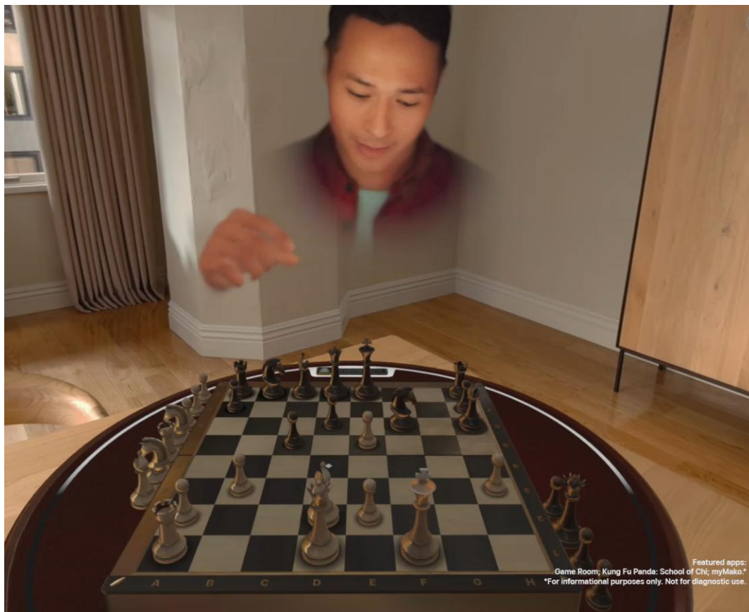
Figure 4: Apple Vision Pro user experience: In AR mode, 3D elements are projected upon the video feed of the real world you are sitting in. This enables Remote Collaborative immersive applications such as a game of chess with another person. The other (remote) person's avatar (realistic 3D scan of their face) and hands are projected real time in your AR space (Apple Vision Pro, n.d.).
