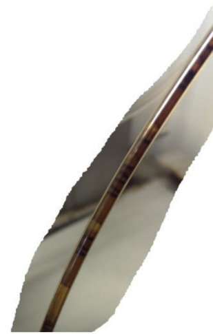
Fig. 12. Fluids at the outlet of the core; appearing more like an emulsion than a foam.
