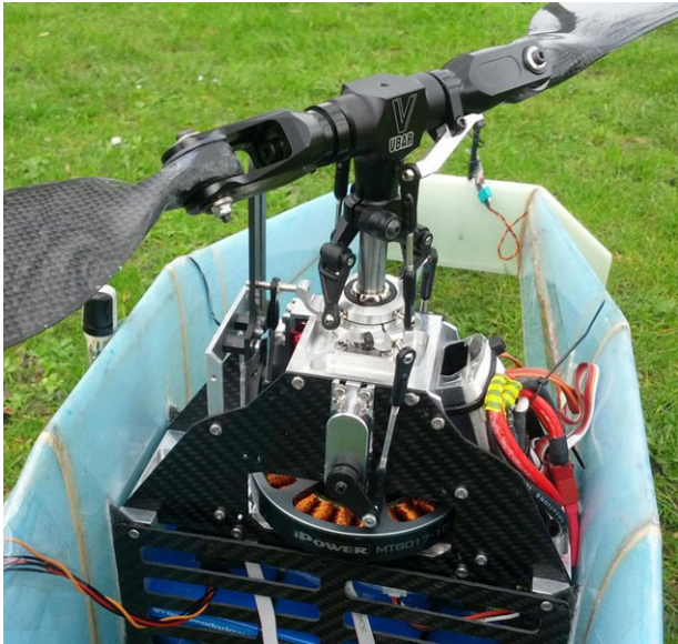
FIGURE 23 Close-up of the rotor head of the DelftaCopter . The swash plate has three gripping points at 120^\circ from each other. The collective pitch can reach from -40^\circ to 40^\circ , which is double that of a conventional helicopter. The self-laminated blades with MA409 section have high camber, a high lift coefficient, and 25 degrees of blade twist from root to tip. Hovering flight is performed at a designed tip angle of attack of around 10^\circ with 1,500 rpm. In forward flight the tip angle of attack can change up to 50^\circ at 500 rpm. The root angle of attack is then about 75^\circ . The blade twist is made possible because the flow is always axial as the DelftaCopter transitions. This allows the rotor to be efficient from hover to fast forward flight
