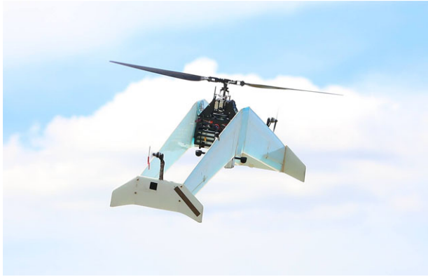
FIGURE 1 Novel hybrid UAV, which combines a cyclic and collective pitch controlled main rotor with a biplane delta wing and torque compensating tip rotors. The biplane concept adds structural rigidity and minimizes the lateral surface area to reduce the perturbations from turbulence during hover. The large main rotor allows efficient hovering flight, whereas the cyclic control provides large control authority in hover
