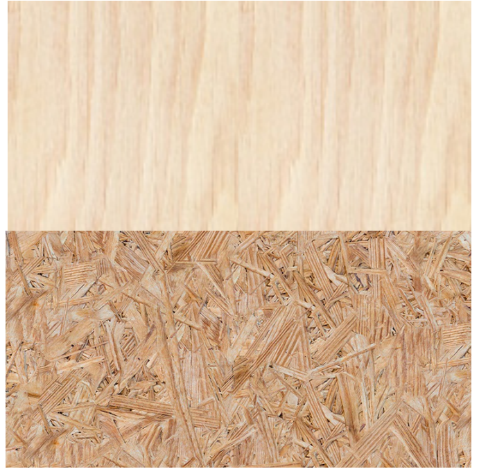
Plywood & OSB plates OSB plates: recycled pressed wood flakes
