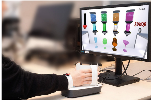
Fig. 2. The portable hand trainer incorporates an actuated compliant shell for grasp training and a passive DoF for pronosupination.
