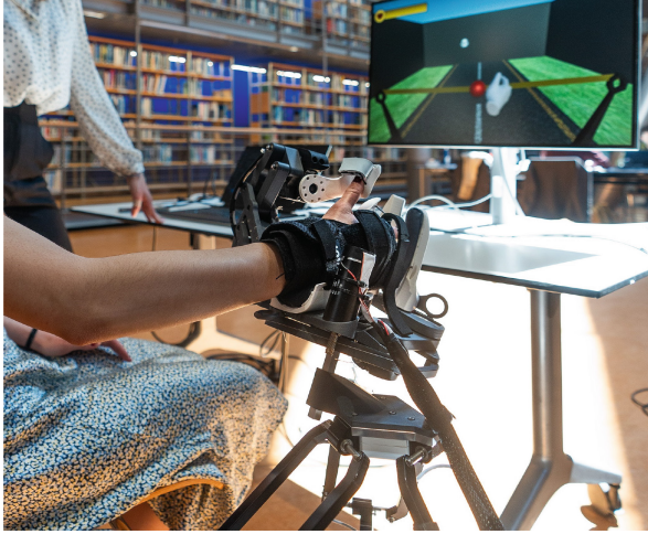
Fig. 1. The Lambda.3+ haptic device consists of a delta robot and a custom hand module for training reaching and grasping movements.
