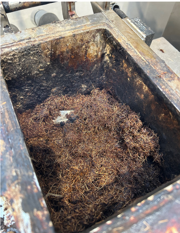
Figure 72. The mixture of N-8040 with flax fibres
