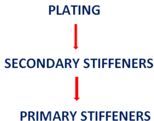
Figure 8 - Structural hierarchy in a ship
