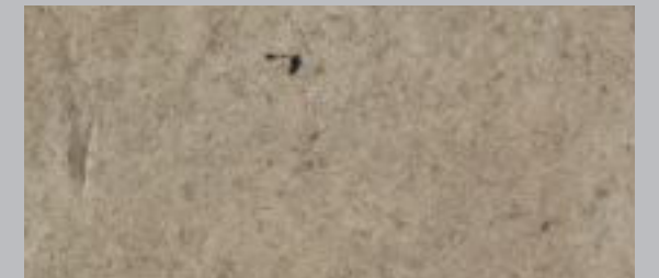
Concrete The second major structural component used is concrete. High strength, fibre reinforced, concrete is used due to the portal construction method and 300mm body width. Poured on site in 2,4x1,5m size. Mix Beige (RAL1001) / Silk Grey (RAL7044)
