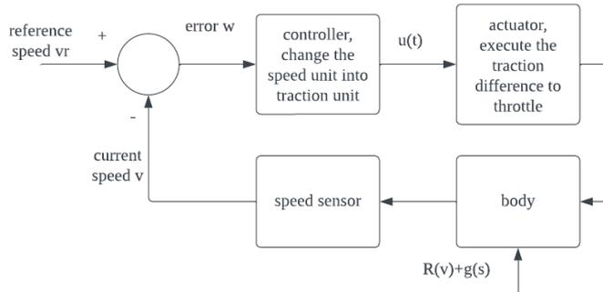
Figure 1: Block diagram of a cruise control system for a train
