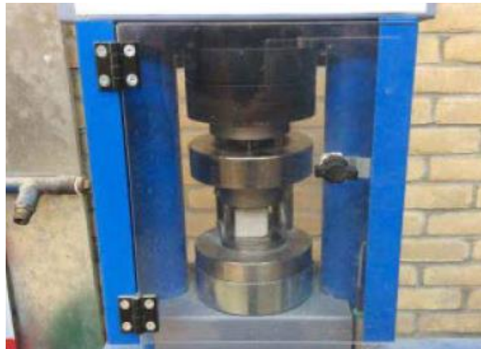
Figure 2.5: Compression test mortar (Esposito et al., 2016 )
