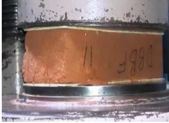
Figure 2.4: Compression test on masonry units (Mishra, 2021 )
