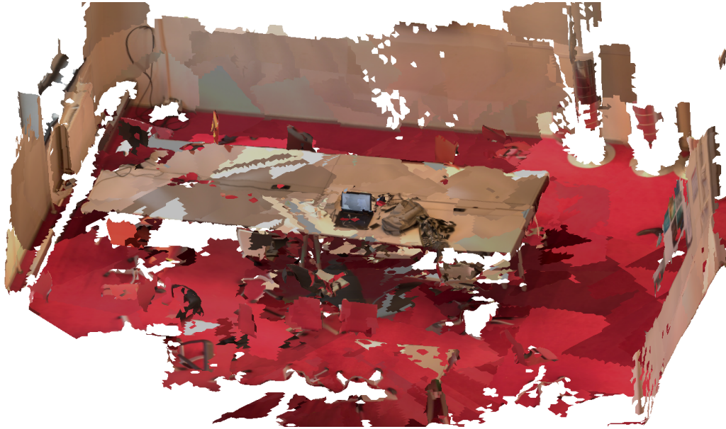
FIGURE 3.9: Polygonal mesh of the scene in FIGURE 3.5 , created on-the-fly.
