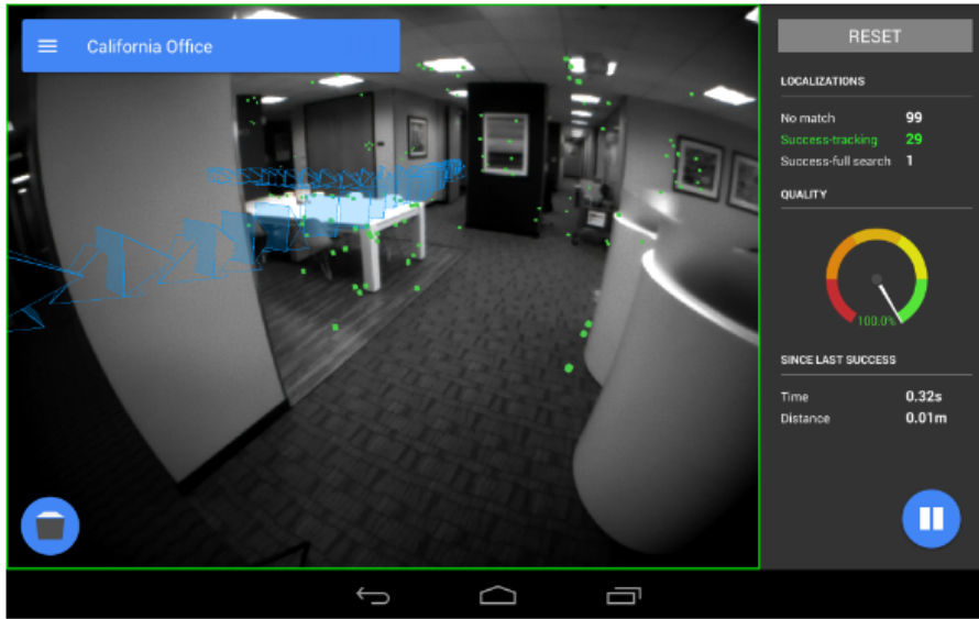
FIGURE 5.3: The interface for a Tango application that would read an ADF and position the user into a known area, for which the ADF was built previously ( Google, 2017b ).
