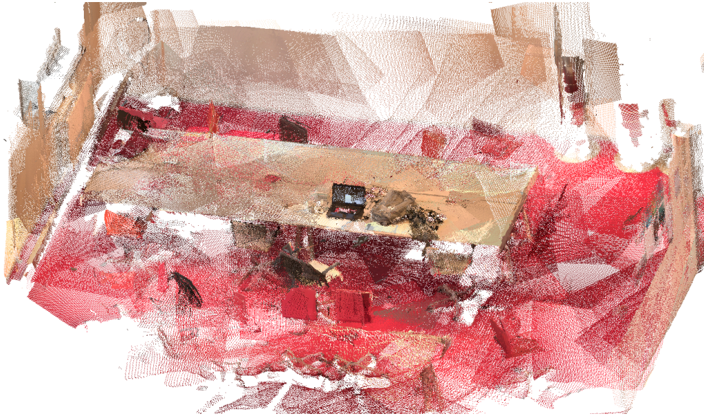
FIGURE 3.5: A frame by frame point cloud created using a VI-SLAM process.
