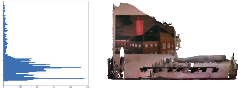
FIGURE 5.6: Side view of the mesh along with its height histogram. The largest bin corresponds to the floor set, and the second to the largest to the table that is located in the middle of the room.
