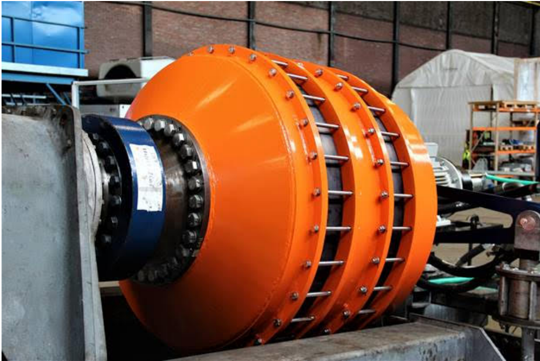
Figure 1.10: A picture of the DOT pump connected to its test bench
