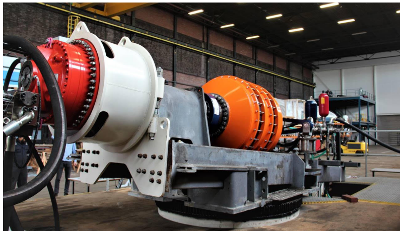
Figure B.1: The DOT pump attached to its test bench
