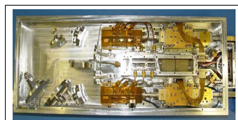
Figure 8. LOA with two multiplication chains, starting from the right with power amplifiers followed by the multipliers (middle) and output optics (left)
