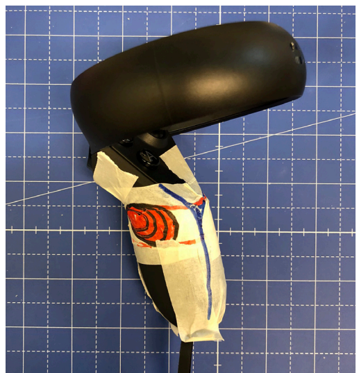
Fig: Physical prototype to determine button changes
