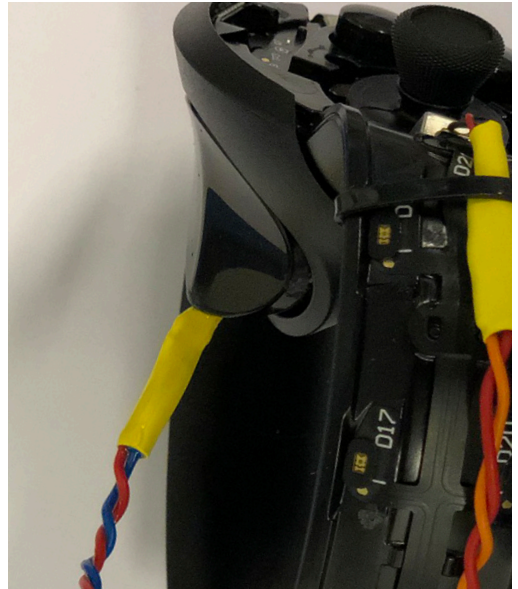
Fig: LRA installed inside Oculus Touch front trigger
