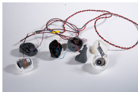
Fig: Trigger prototypes with various actuator orientations and actuators.
