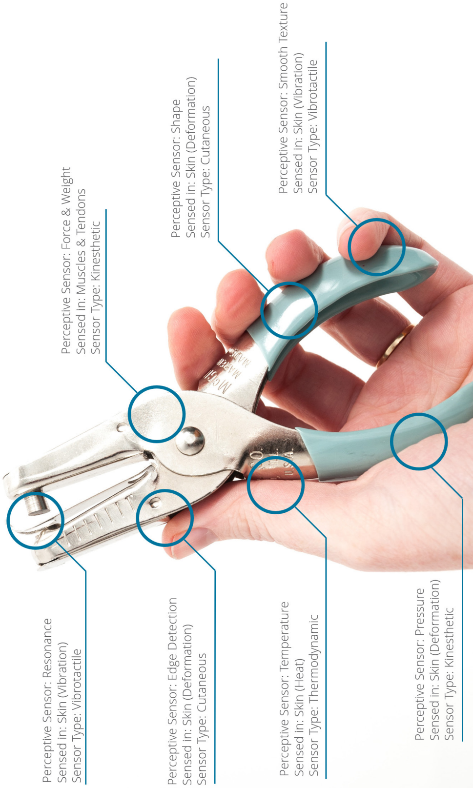
Fig: Different aspects of touch as shown through a hole punch interaction.
