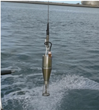
Figure 2.8: In situ device for measuring the yield stress (Rheotune).
