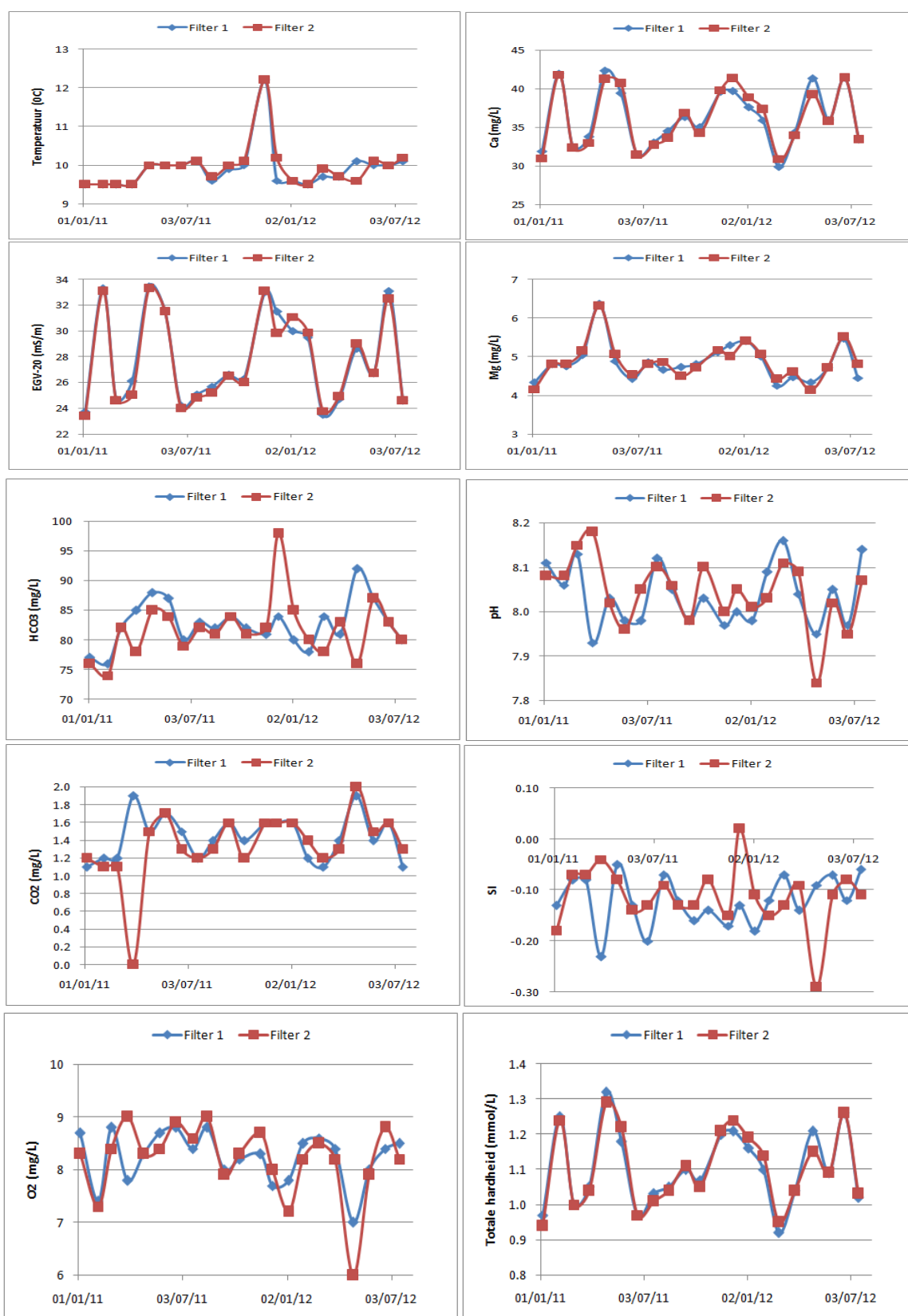
Figure 66: Measurements of post-filtrated effluent at Honderloo
