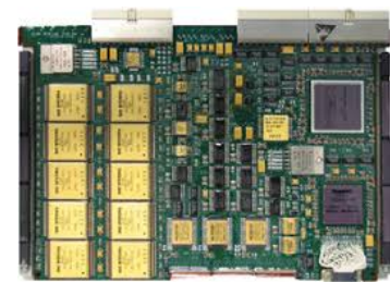
Figure 12.2: RAD750® 6U CompactPCI Single-Board Computer produced by BAE Systems.
