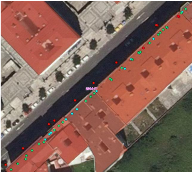
Figure 14. Location of step and ramp entrances. Colour code: buildings in semi-transparent red, step entrances in green, ramp entrances in blue and tree gratings and entrance errors in red.
