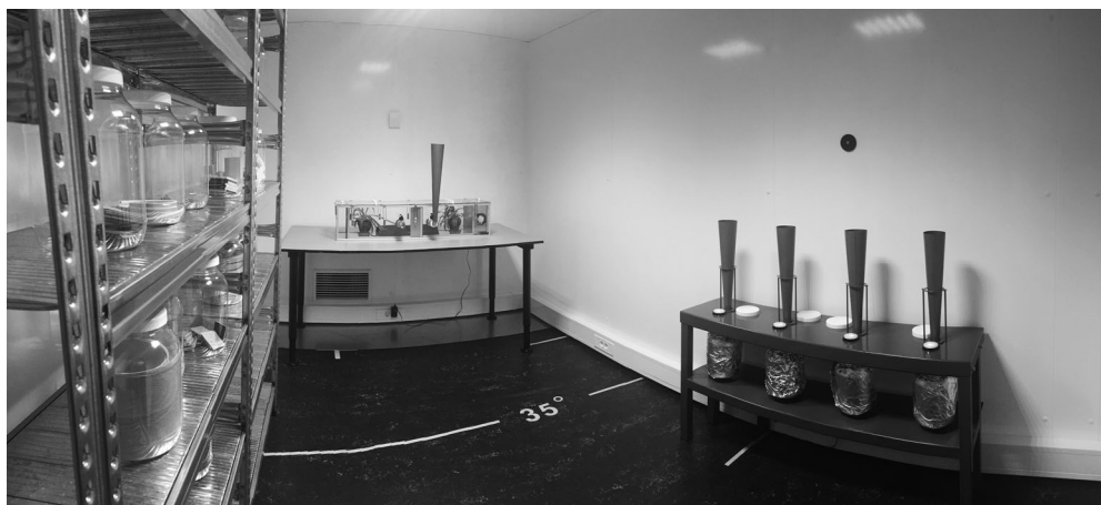
Figure 1. Air Quality Chamber: CLIMPAQ 50L and sniffing table.
