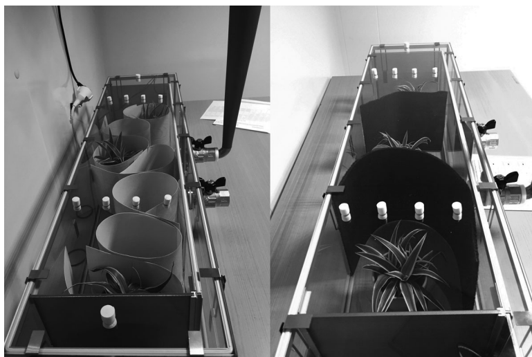
Figure 3. Selected materials + Spider plant inside of the CLIMPAQ 50L.
