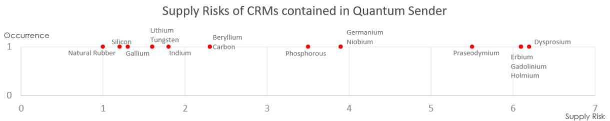
Figure D3.2: Supply Risks of CRMs contained in Quantum Senders.
