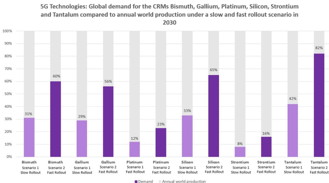
Figure 6.3: 5G Technologies: Global demand for the CRMs Bi, Ga, Pt, Si, Sr and Ta compared to world annual production rates under slow and fast rollout scenarios in 2030.
