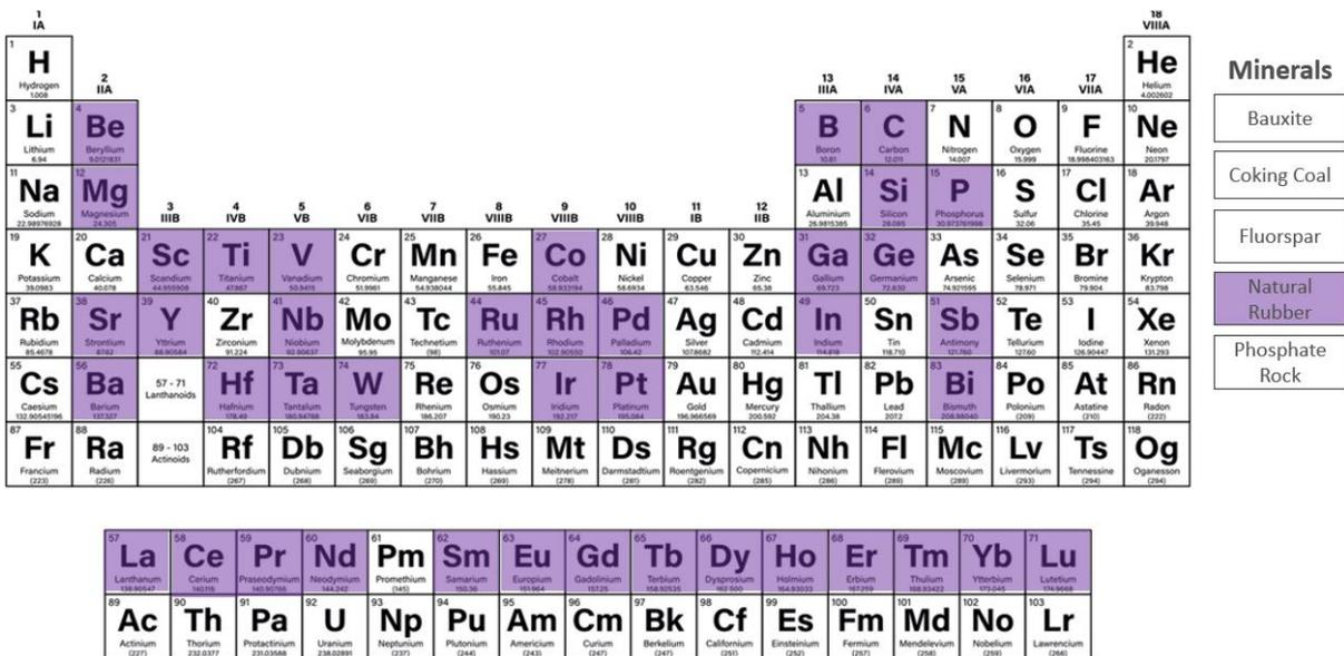
Figure 4.4: Critical Raw Materials contained in 5G Technologies.
