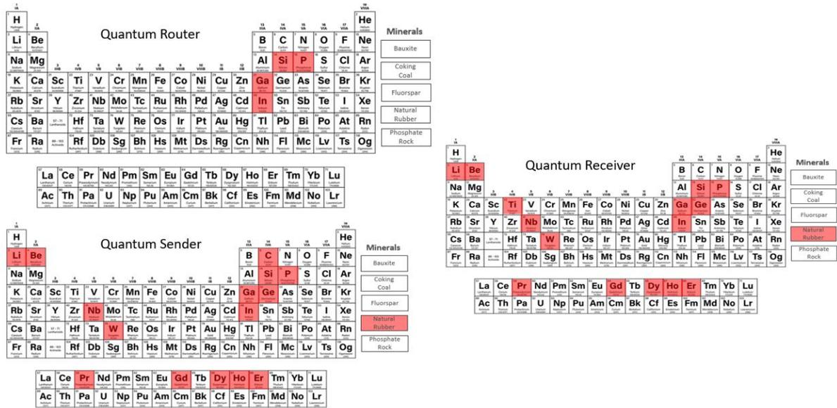
Figure 4.11: Critical Raw Materials contained in the different Quantum Devices.
