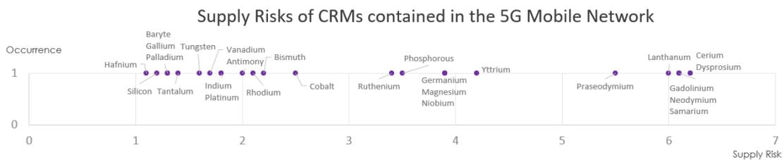
Figure A2.2: Supply Risks of CRMs contained in the 5G Mobile Network.
