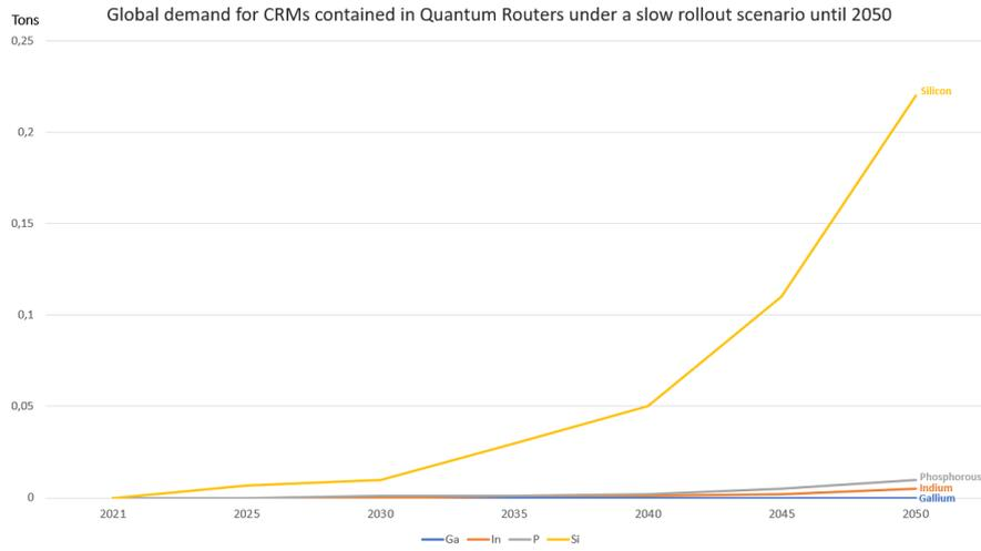
Figure J2.1: Demand development for CRMs contained in Quantum Routers under a slow rollout scenario until 2050.
