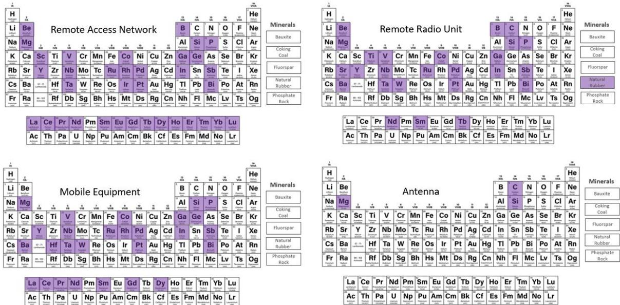
Figure 4.3: Critical Raw Materials contained in a 5G Equipment.
