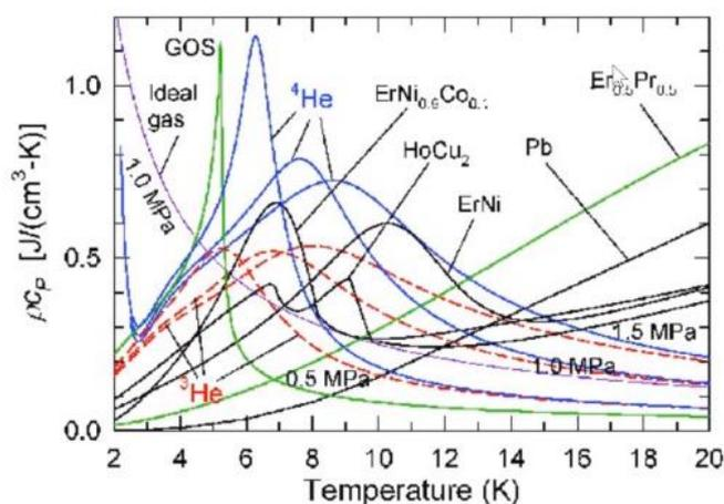
The diagram shows the heat capacity and volume temperature. If the curves are going down, this means that the properties decline, which makes it less useful for cryogenics. Furthermore, in order to use cryogenics, it has to be cooled to very low temperatures, between 2,7K and max. 10K. In order to unite these properties, solely the following materials can be potentially used:
