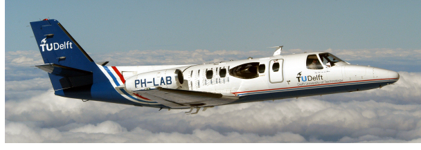
Fig. 1 CS-25 class Cessna 550 Citation II PH-LAB research aircraft operated by the Delft University of Technology.
