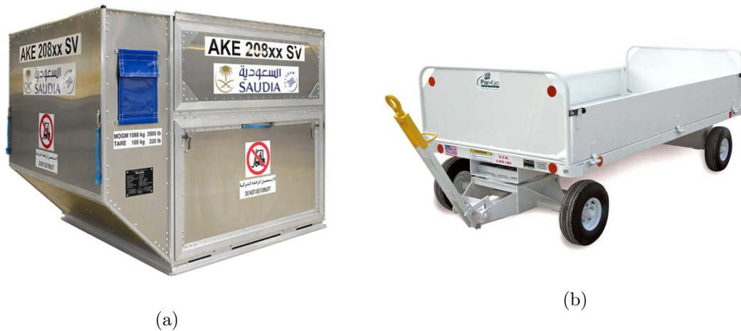
Figure 4.6: Examples of a baggage ULD (a) and baggage container (b) (VRR, 2018; AERO Specialities, 2018)
