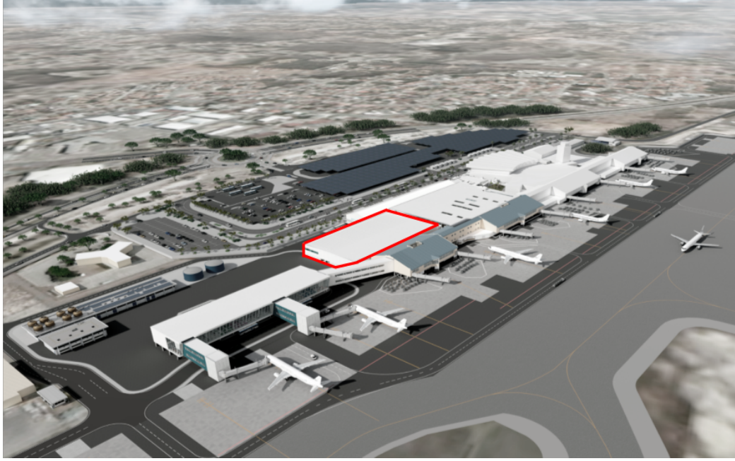
Figure 6.3: The new terminal layout of AUA with the new BHS building highlighted in red
