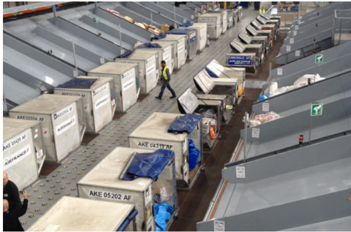
Figure 4.8: A non-driven ALT system at Paris-Charles de Gaulle airport (Aircargonews, 2015)
