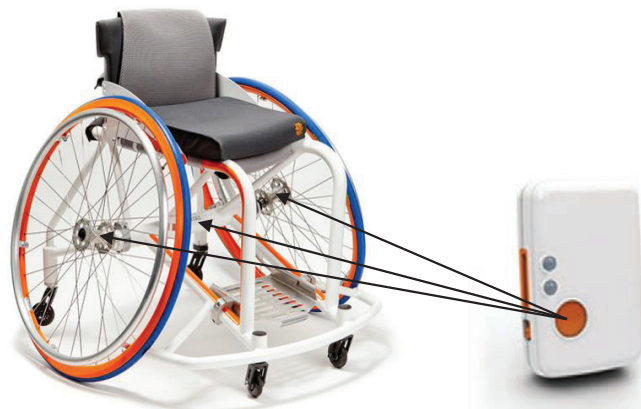
Figure 1: Sensor mounting locations on the wheelchair
