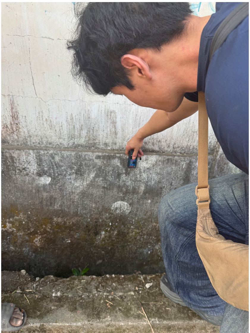
Measuring visible floodline on the wall
