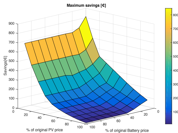
Figure 56 Maximum saving with 2.0A under different PV/battery prices
