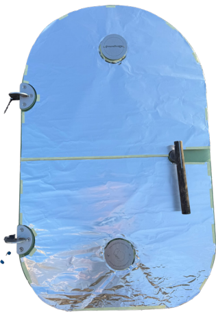
figure 5.2.3.1: Aluminium plate on GF door. Source: author
