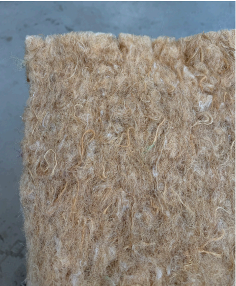
figure 3.7.1: Flax wool insulation. Source: author
