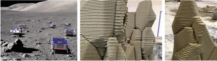
Fig. 1. Rhizome 1.0 1 prototypes using TU Delft rovers (left) and Vertico's cement-based concrete and robotic system (right)
