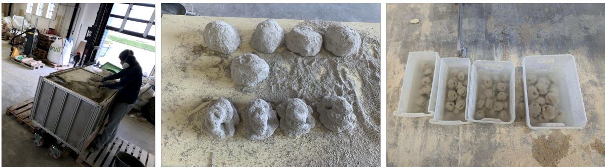
Figure 3.5: Different stages of the cleaning process: a) excavation of the elements from tray, b) removal of excess cement material, c) curing with water
