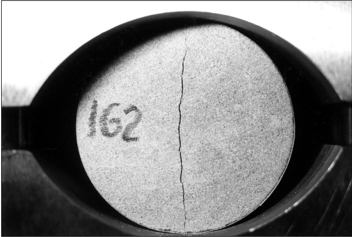
Figure 1-43: A BTS test after failure.
