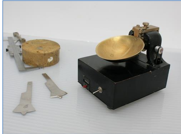
Figure 1-20: Liquid limit device.
