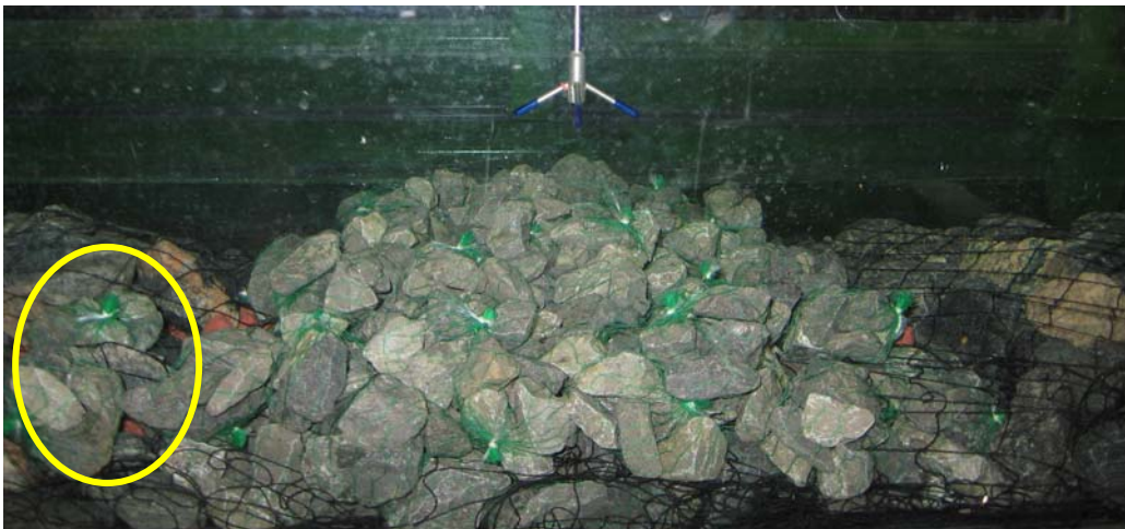
Figure 4.6: Test setup just after occurrence of incipient motion
