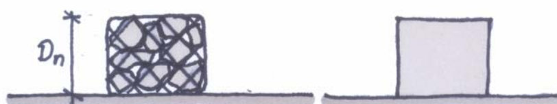
Figure 2.4: Cube shaped box gabion and same size cube shaped rock with lower \Delta
